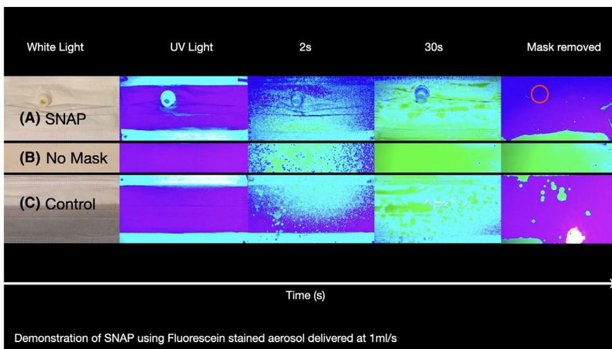
**FIGURE 2** In Vitro Aerosolised Fluorescein test results 1ml/s through a 50 micro point. From superior to inferior: (A) “mask fitted with SNAP” vs. (B) “no mask” vs. (C) “mask with no SNAP” as positive control to demonstrate no leakage through the mask material. No visual difference seen and no leak through the SNAP valve (red circle)
