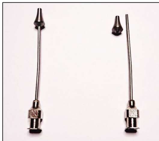
Fig. 1 Showing visual of the defect noted above
